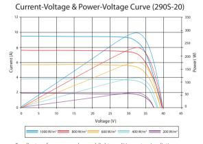
Excellent performance under weak light conditions: at an irradiation intensity of 200 W/m<sup>2</sup> (AM 1.5, 25 °C), **98%** efficiency (200 W/m<sup>2</sup> ) is achieved
